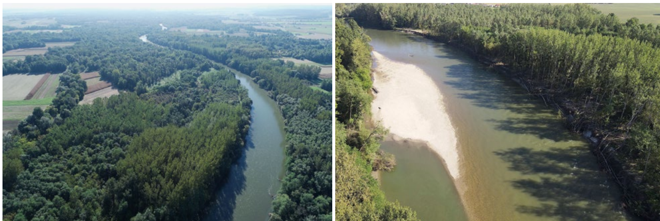
Figure 3. A section of the Mura River near the village of Petanjci. On the left side, in 2022, the river is very regulated and doesn't have much space. Only one year later, after the implementation of the measures of the Natura MURA project, in this case, the widening of the river bed, the river takes a more natural shape and has more space to form vital habitats such as sandbanks and gravel islands as shown in the photo on the right side. ©VGP, Simon Veberič
