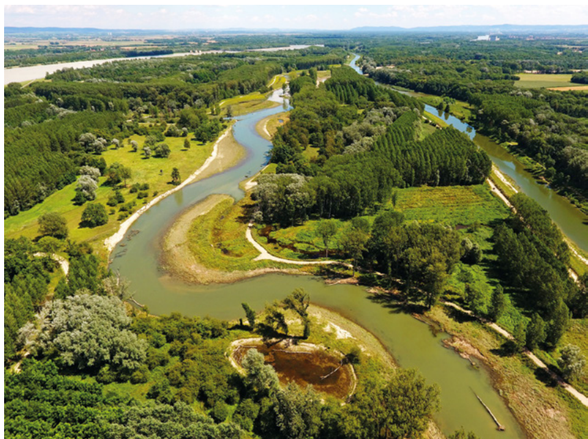
Figure 1. The sinuous course of the New Traisen within the newly lowered floodplain corridor. On the right is the straight former Traisen canal. In the background is the Danube with its surrounding floodplain forests (© Pock/VERBUND).
