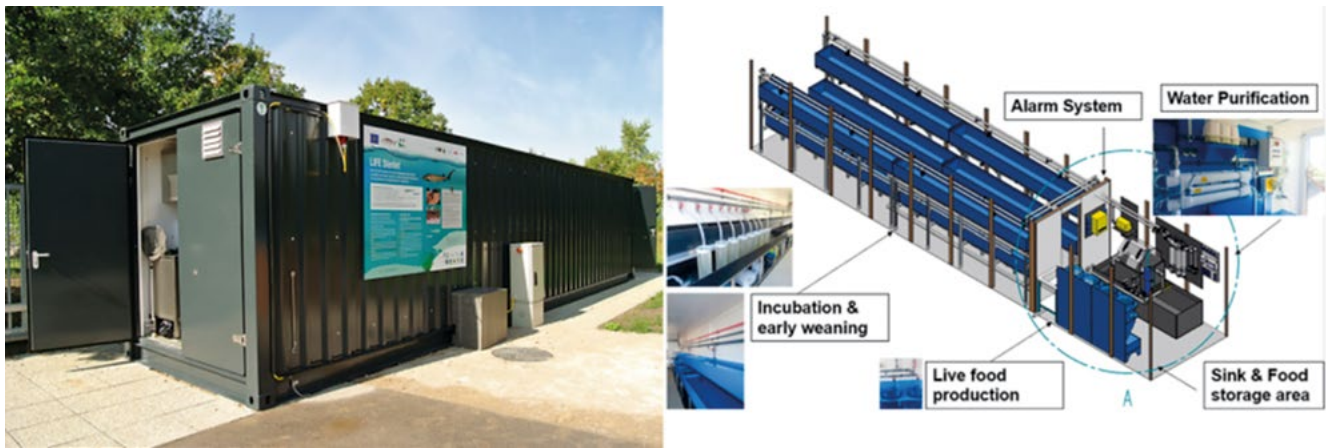
Figure 1. The hatchery container: left - outside view; right - technical sketch
