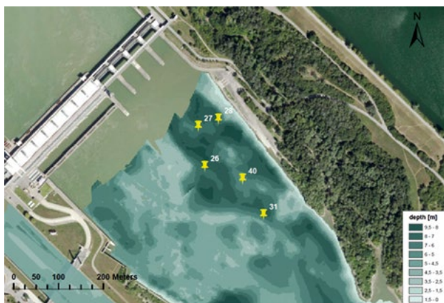
Figure 3. Hydrophone positions of the 2D- telemetry study
