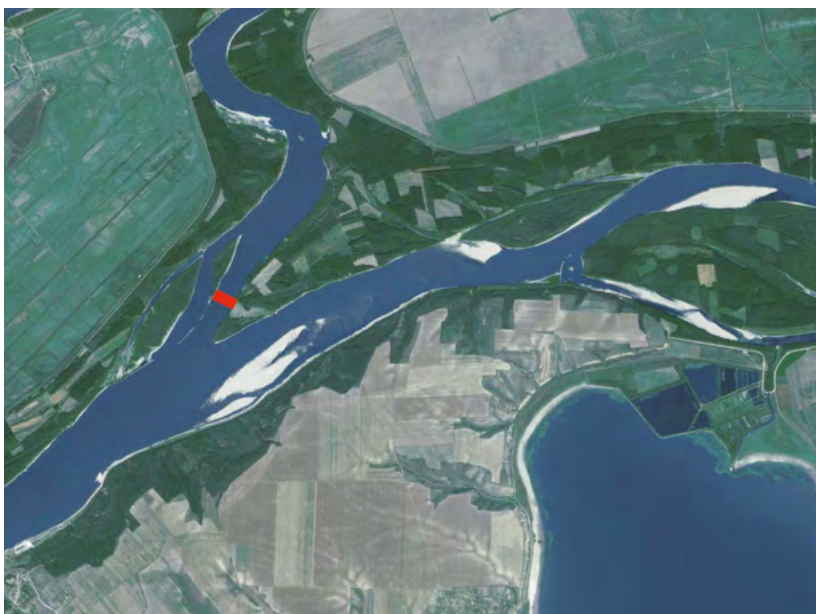
Figure 2. The bifurcation Bala Branch – Old Danube near Braila. The partly constructed submerged sill in the Bala Branch (red line) and the guiding wall along the left bank have increased the local flow velocity and, consequently, the erosion of the river bottom. Only few sturgeons could occasionally pass the sill and spawning migration is disrupted. Presently, alternatives are being evaluated (Source: AFDJ, Galati, WS 7 October 2015)
