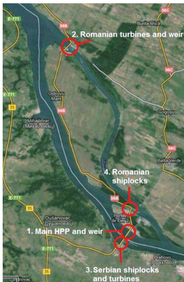
Figure 1. The Iron Gate Hydropower dams. While the Iron Gate I dam (left) is a single obstacle, the situation at Iron Gate II (right) is extremely complex with two hydropower stations and two ship locks (Sources: Photo Jürg Bloesch; de Bruijne et al. 2014)
