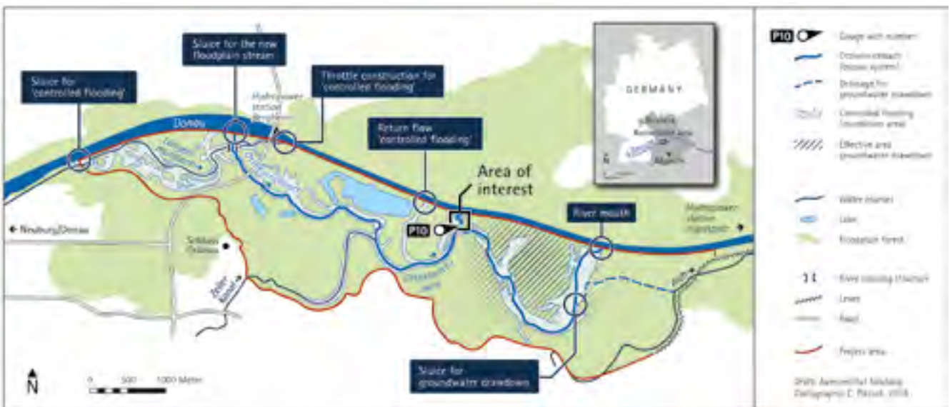
Figure 1. Simplified map of the study area and location of the measures (new floodplain stream, controlled flooding and groundwater draw-down) and the area of interest with gauging station "P10" for water level measurements
