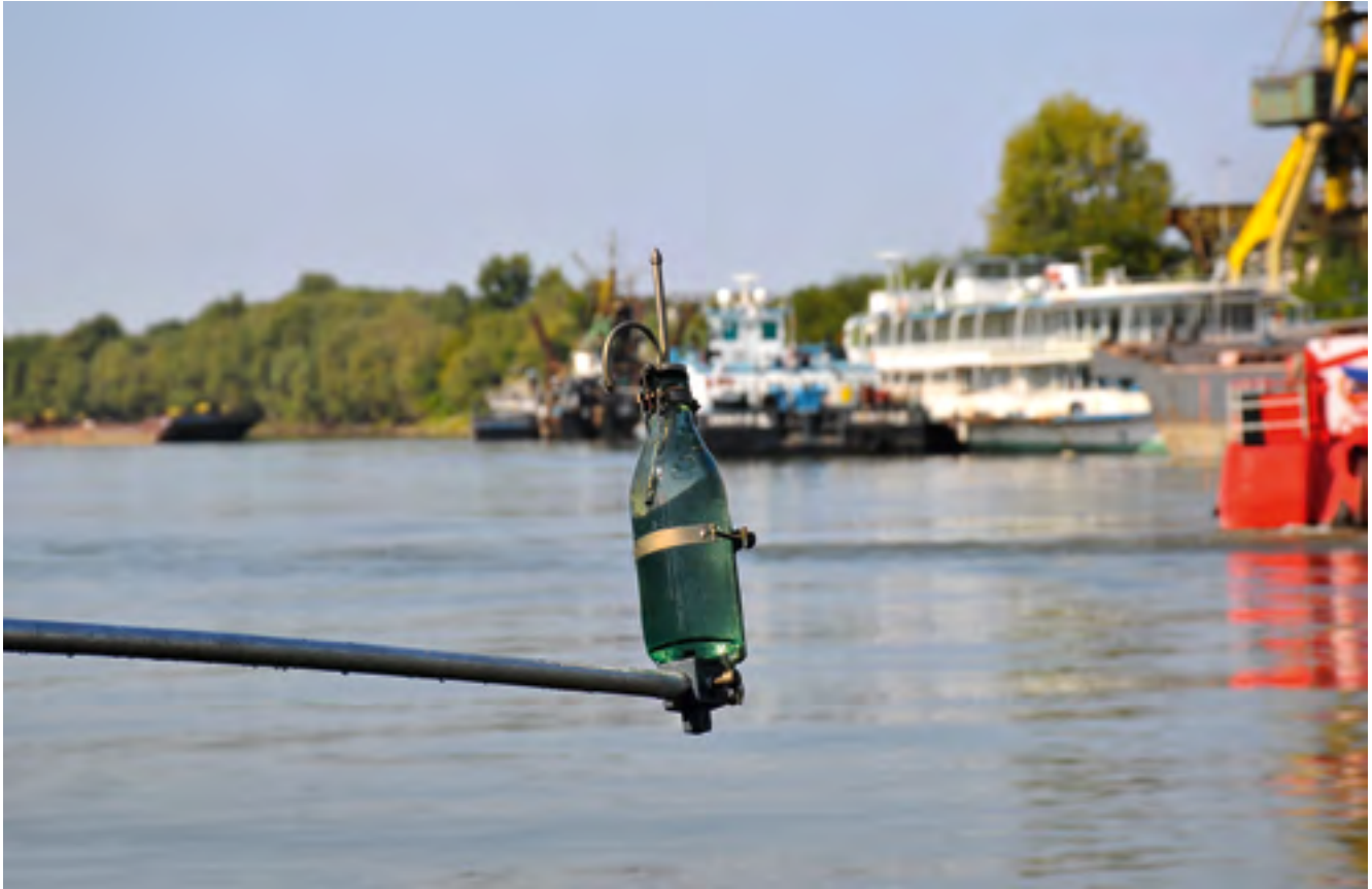
Figure 3. Sampler in Bulgaria using the depth-integral method. Source: Marlene Haimann / IWHW – BOKU
