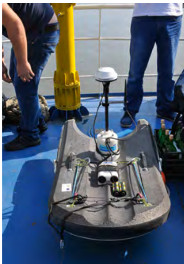
Figure 2. An Acoustic Doppler Current Profiler measures flow velocity and water depth, which are needed to calculate the discharge in a cross section. Source: Marlene Haimann / IWHW – BOKU
