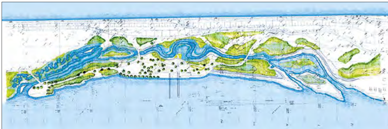
Figure 3. Near natural fish bypass system Freudenuau (Waidbacher)
